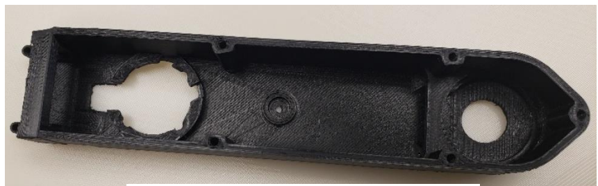
Figure 4.5 3D printed upper leg shell [2]
