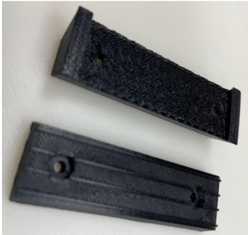
Figure 4.10 3D printed upper and lower links for tread
