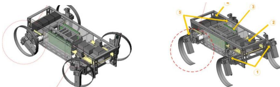
Figure 3.1. Computer aided design (CAD) drawings of robot operating in wheel (left) and leg (right) modes (10)
